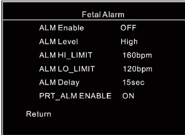
Alarm Enable: Whether enable fetal parameter out-of-limit alarm; ON --- Enable; OFF --- Disable.
