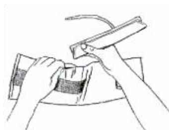
Fig. 8-3 Replacing Rubber Bags in the Cuff
