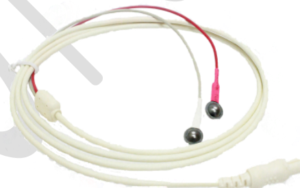
Fig 1-5A Connection cable of EOG, EMG Nr 1: Record Side; Nr 2: Reference side.
