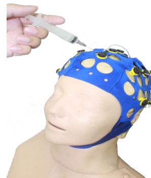
Fig 3-2 Applying EEG gel on the electrodes of EEG cap worn by a subject
