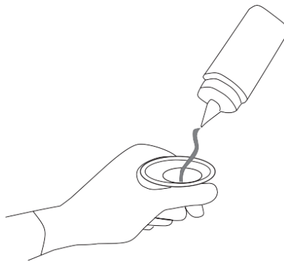
Figure 45 Add Coupling Gel into the Probe Sheath
