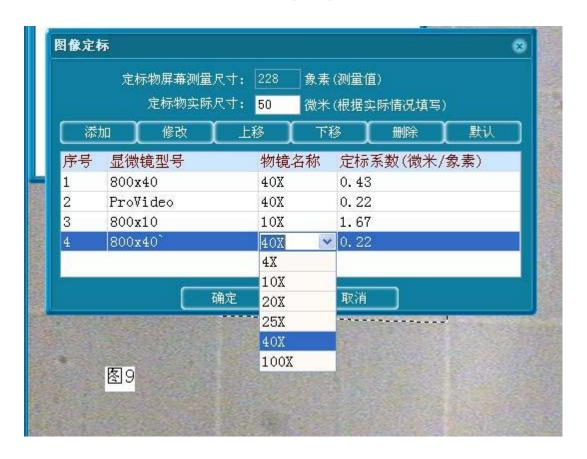
Fill the previous measurements (ant line) of the paragraph above in the window "Actual Size of the calibration substance" column, the physical length of the border box (the actual side length of the grid in standard count pool is 250 um; the small grid is 50 um). Then click the "Add" button to add a line of calibration item.
